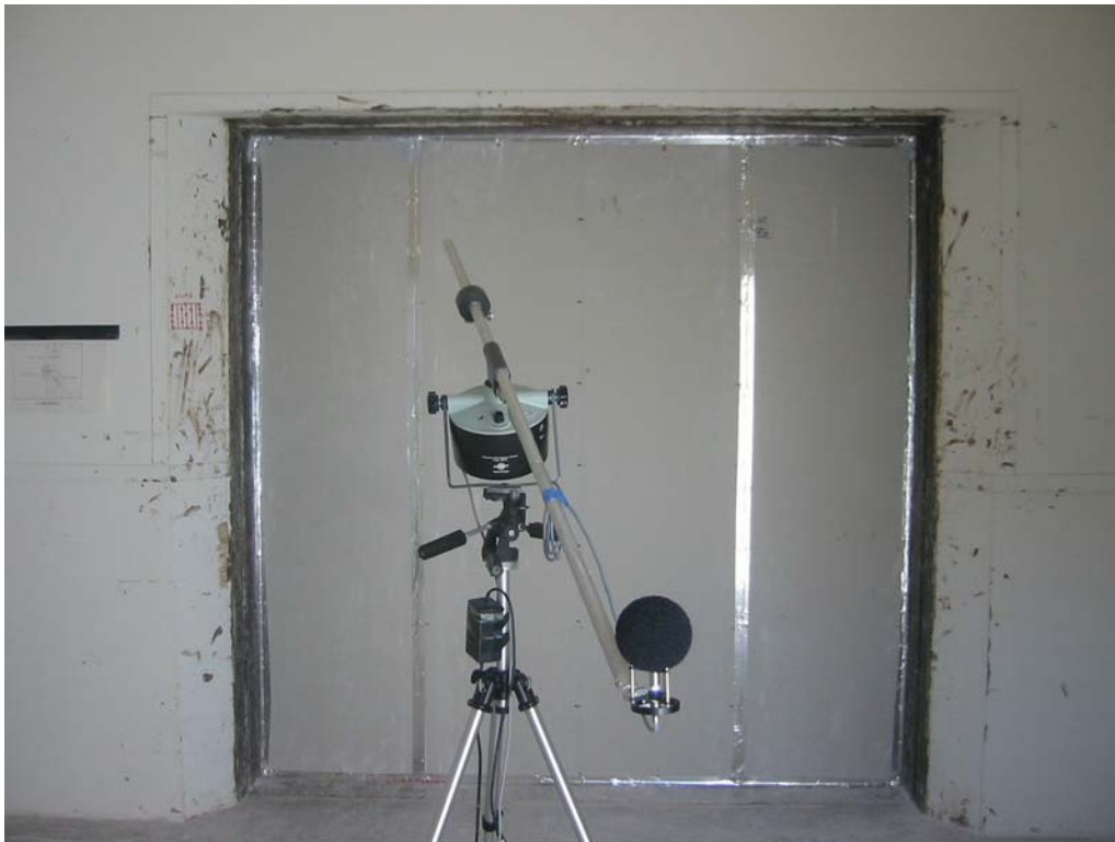
Figure 1: Photograph of typical staggered seam pattern on source room side of partition
