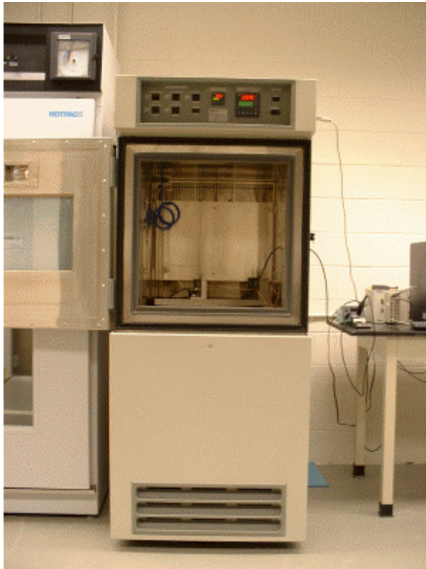
Figure 5: Environmental Chamber Utilized for Vibrating Beam Technique Data Acquisition
