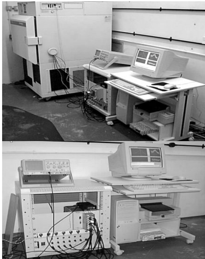
Figure 4: VBT System – Vibrating Beam Technique Data Acquisition Hardware
